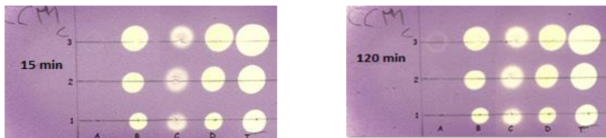
Figure 1: Image of the silica plate showing the different extracts of Origanum elongatum and Cupressus atlantica after 15 and 120 min of reaction with the DPPH at 6.10 -5 M. Cupressus atlantica : A: Essential oil B: Organic extract. Origanum elongatum : C: Essential oil D: Organic extract. T: \delta -Tocopherol at 0.4 mg / ml. Volumes deposited 1: 2 \mu l, 2: 4 \mu l and 3: 8 \mu l
