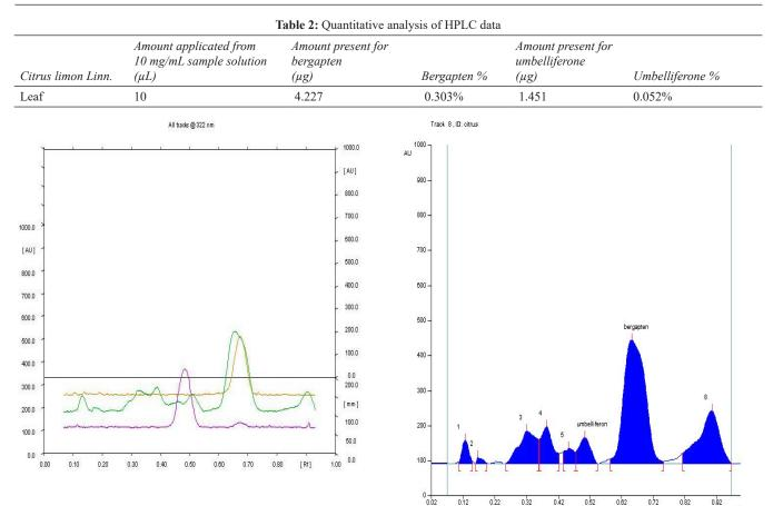
Figure 1: Chromatographic profile of std. and sample *C. limon*; UM: umbelliferone; BR: bergapten; LV: leaf
