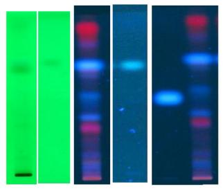
**Figure 4:** HPTLC fingerprinting profile of *C. limon* Linn. at 254, 366 nm; LV: leaf; UM: umbelliferone; BR: bergapten
