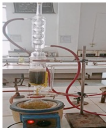
Figure 3 : Extraction of leaves using Hot Continuous Percolation method by Soxhlet apparatus and by Maceration method
