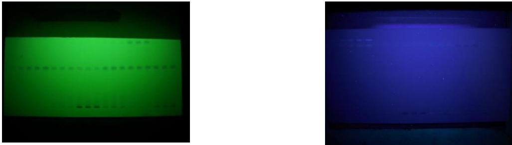
Figure 5: Elution of \alpha -mangostin standard and samples using chloroform : ethyl acetate (85:15) v/v on silica gel F 254 (a) identification by UV 254 (b) identification by UV 366 .
