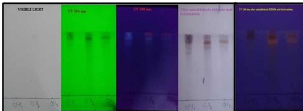
Figure 1: TLC of Chloroform: Ethyl acetate fractions (CEF 1 , CEF 2 and CEF 3 ) showing flavonoids, phenolic acids and glycosides.
