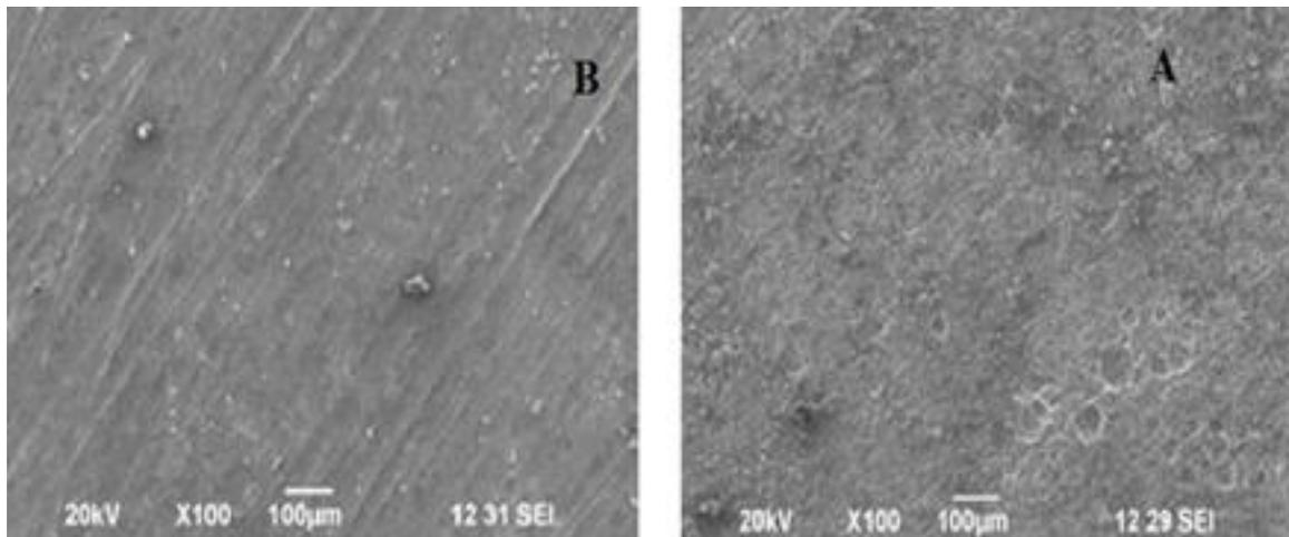
Figure 4: SEM images of MS in 1 M H<sub>2</sub>SO<sub>4</sub> media (a) and (b) with Zygophyllum album extract (1400 ppm).
