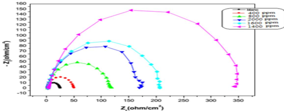
Figure 3: Nyquist plots showing effect of Zygophyllum album extracts on corrosion of MS in H<sub>2</sub>SO<sub>4</sub> medium.
