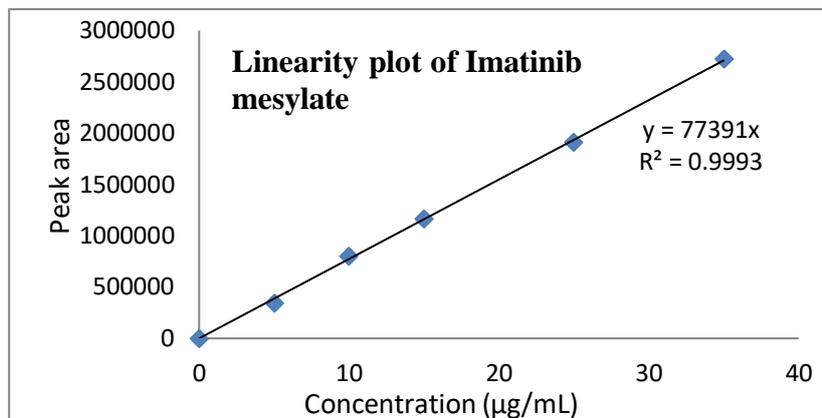
Figure 5: Linearity plot of Imatinib mesylate.
