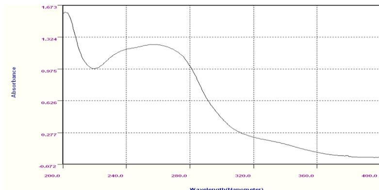
Figure 4: UV spectrum of Imatinib mesylate.
