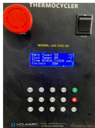
Figure 5. Control panel of the thermocycler showing temperature range and cycling parameters.
