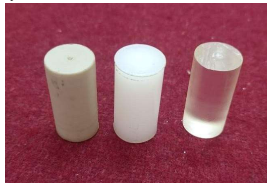
Figure 1: Specimen of size 15 mm by 30 mm size for Shore hardness test and Compression test for peak stress.
