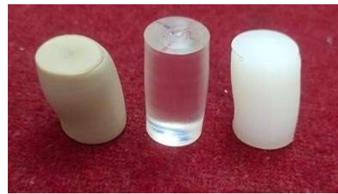
Figure 5: Specimen after compression test
