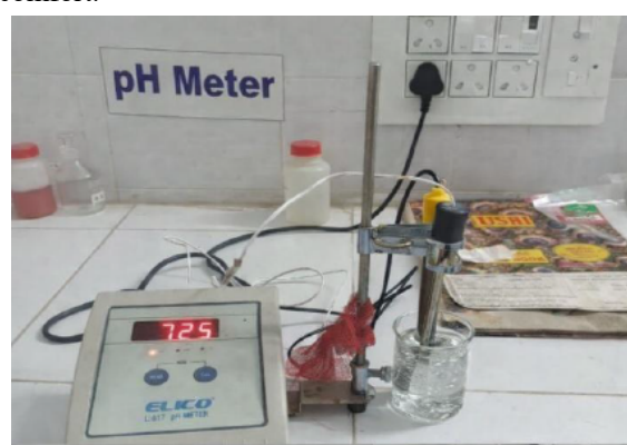
Fig 8. pH measurement of Optimised F3 formulations
