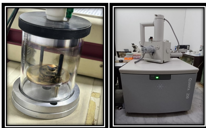
Figure4: (a) Gutta percha cones placed for gold plating, (b) Scanning electron microscope
