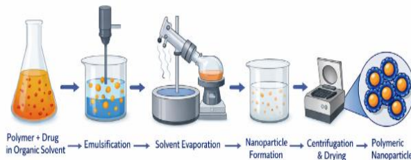
Figure 2.1: Schematic representation of polymeric nanoparticle preparation using solvent evaporation method
