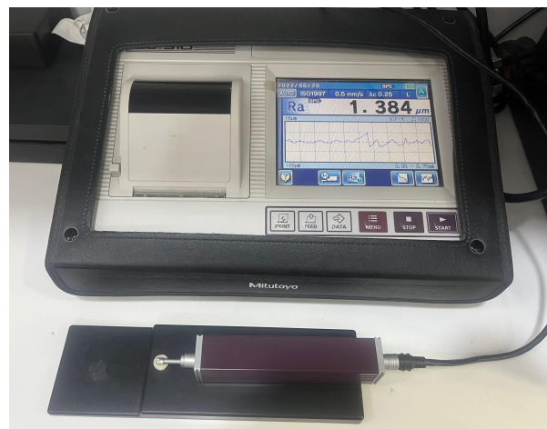
Figure 1: This picture represents a stylus profilometer
