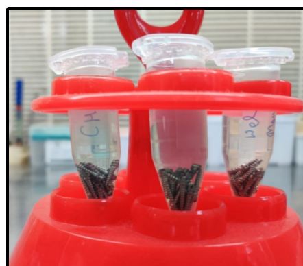
Fig 2: Preparation of eluates from Mini screws in different types of mouthwash.
