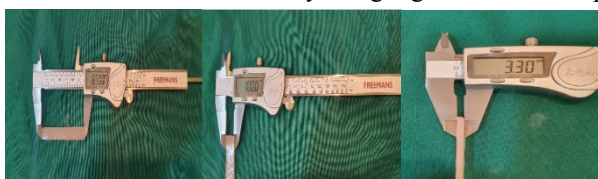
FIGURE 6: MEASUREMENT OF DIMENSIONS OF RECTANGULAR SHAPED SPECIMENS
