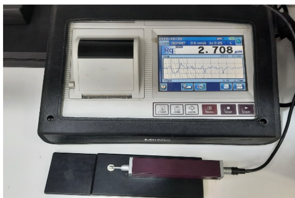
Image 1: Measurement of surface roughness using Stylus profilometer
