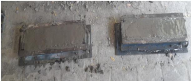
Figure 7.2: Casting of beams
