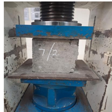
Figure 7.1: Testing of Concrete cubes
