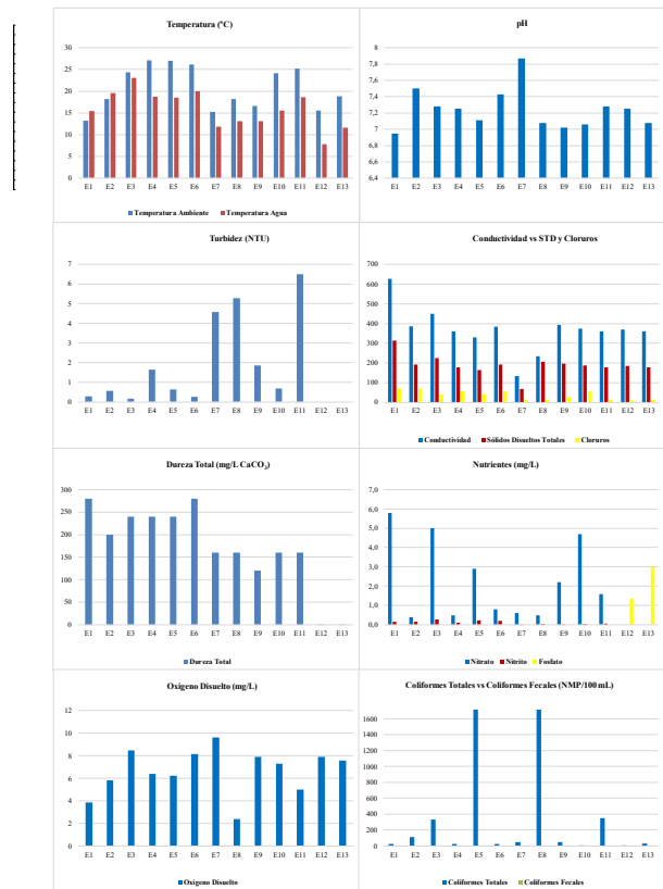
Figure 3. Graphic representation of the physicochemical parameters of the water quality of the Locality of Colliguay, Valparaíso Region.
