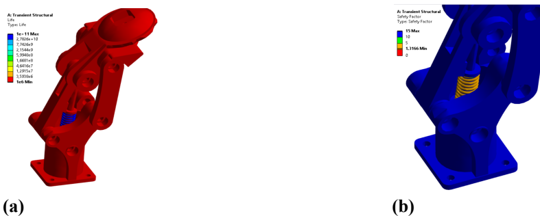
Figure 12. Results of the spring fatigue simulation: (a) Number of cycles the spring will withstand under cyclic loading 1 \times 10^{11} cycles; (b) Minimum safety factor of the fatigue spring of 1.3166.
