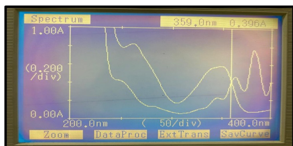
Figure 3: Overlay spectra of BBR and AMB with an intersection point at 359.0 nm
