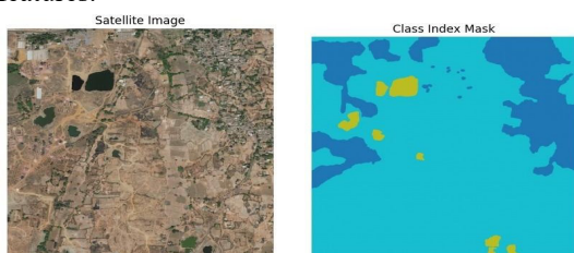
Fig. 10. Original satellite scene and its generated class index mask representing land cover categories.
