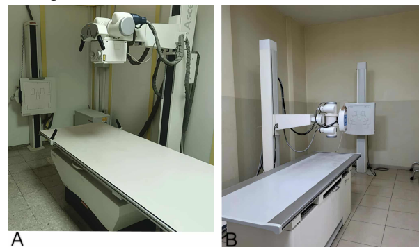
Figure 1: The image show the X-ray devices used in the evaluation of radiation dose during patient examinations. A) showed Carestream DRX-Ascend; DRX Plus detector, B) JPI Healthcare – DR system.
