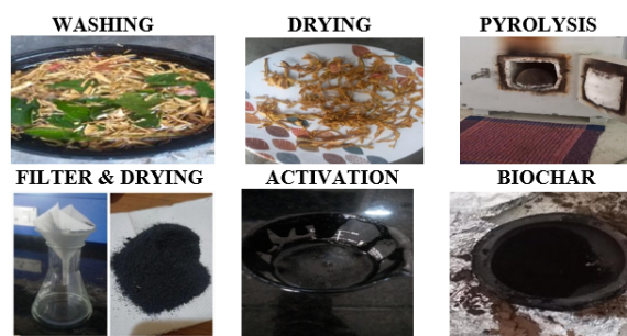
Fig 1: Flowsheet of preparation of biochar adsorbent.
