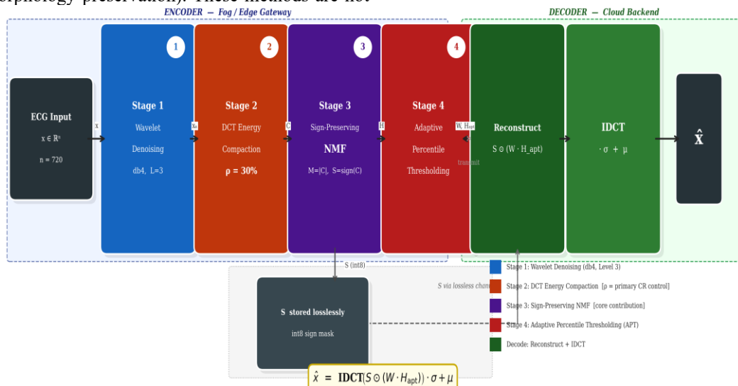
Fig. 1. LEC-Wave-TFT four-stage encoder–decoder architecture. Stage 1: Wavelet denoising (db4, Level 3); Stage 2: DCT Energy Compaction ( \rho=30\% , primary CR control); Stage 3: Sign-Preserving NMF (core contribution; M=|C|, S=\text{sign}(C) ); Stage 4: Adaptive Percentile Thresholding (APT, 50th pct). W is learned offline on calibration data and frozen. S is transmitted losslessly as int8. Reconstruction: \hat{x}=\text{IDCT}(S \odot (W \cdot H_{\text{apt}})) \cdot \sigma + \mu .
