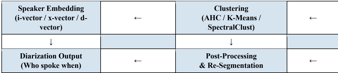
Fig. 1. Traditional Speaker Diarization Pipeline (Modular Cascade)
