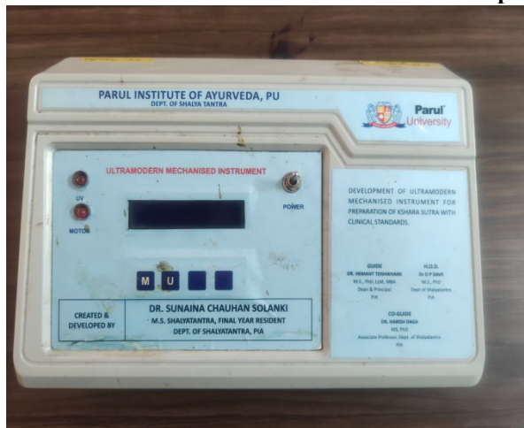
Figure (I) - Electronic Control Unit With Switches & LCD Display And LEDs:
