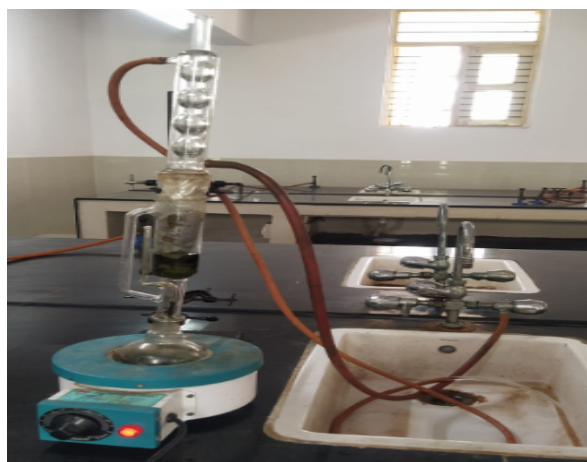
Fig. 1 Soxhlet Extraction Process
