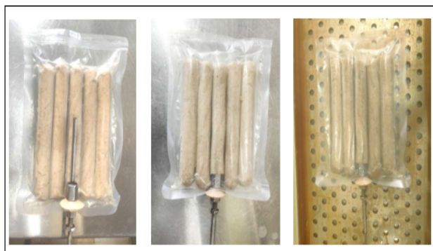
Figure 1. Packed plant-based sausages on retort tray with probes
