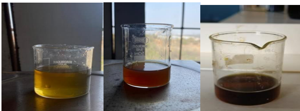
Fig. 2 (a) Aqueous leaf extract (b) Leaf extract with Ferric nitrate solution (c) Synthesized INP Solution
