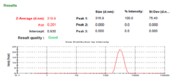
Figure 3 Particle size distribution and morphology of synthesized MSNs
