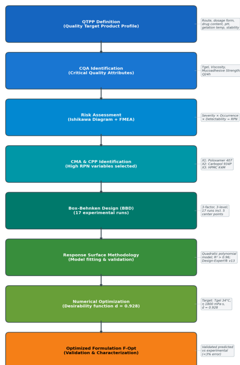
Fig. 1. QbD framework workflow applied in the development and optimization of the rutin-loaded mucoadhesive in situ hydrogel.
