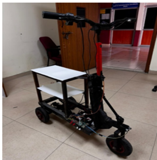
Fig 2 - Three-wheeled autonomous electric vehicle prototype used for experiments
