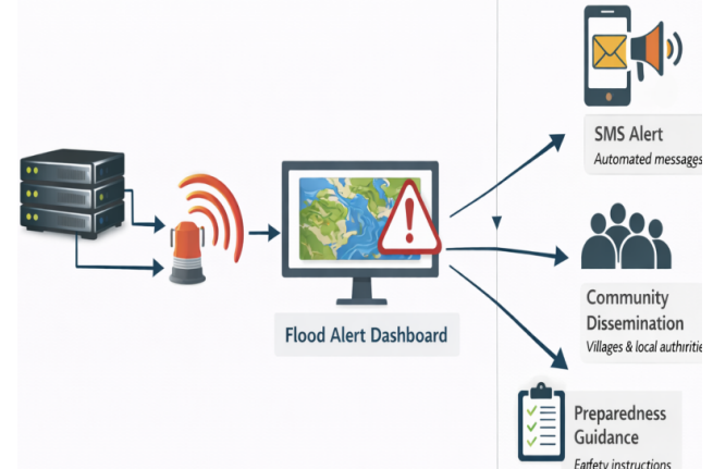
Fig 2: Flood alert dissemination flowchart
