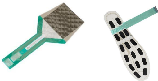
Fig 3: Minimally invasive high resolution sensor AND 4Foot pressure[3]
