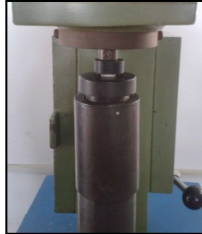
Fig 5: A static load of 15 kg was applied on the top of glass plates
