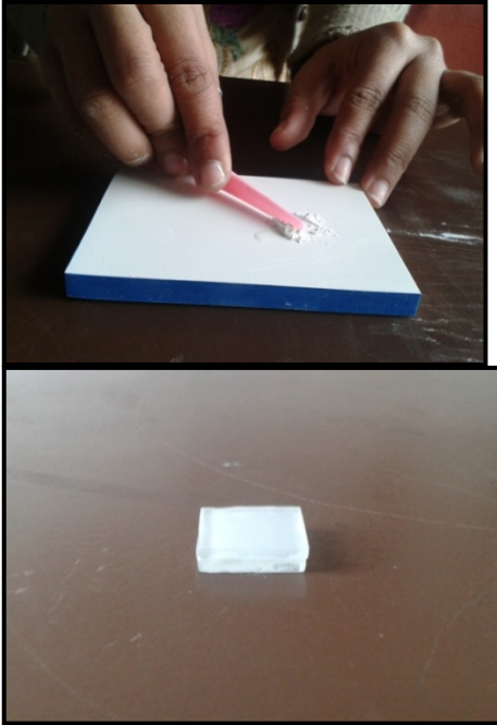
Fig 3: Mixing of glass ionomer powder Fig 4: The cement was placed between a pair of glass slab of uniform thickness
