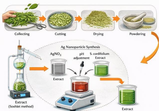
Figure 3: Visual color change during green synthesis of silver nanoparticles using plant extract.
