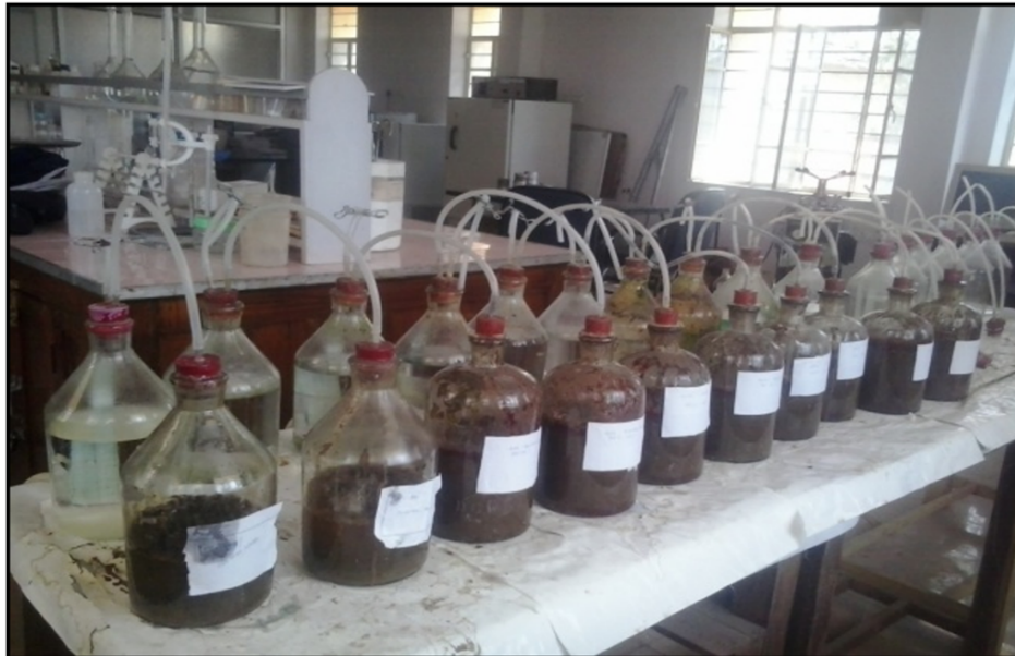
Fig. 1: Laboratory experiment for bio-methanation
