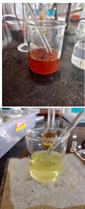
Fig.1: (A) Reddish color of Fe 3+ (B) change in color of Fe 3+ to green Fe 2+
