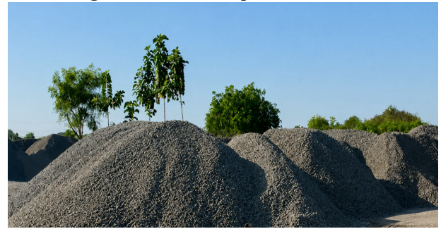
Figure 3. Recycled coarse aggregate (RCA) sourced from demolished structural concrete
