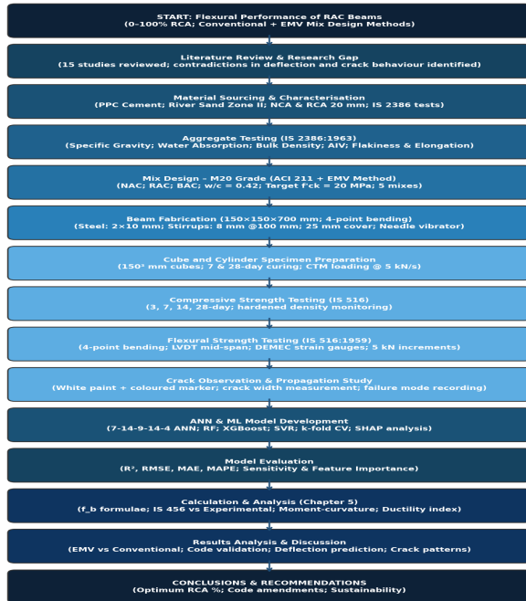
Figure 1. Research methodology flowchart: from material characterisation and mix design through experimental testing to ANN model development and SHAP feature importance analysis.
