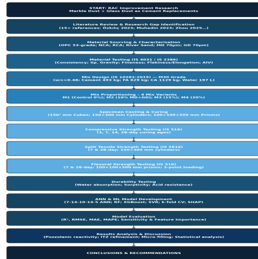
Figure 1. Research methodology flowchart: from material characterisation through experimental testing to ML model development and analysis.
