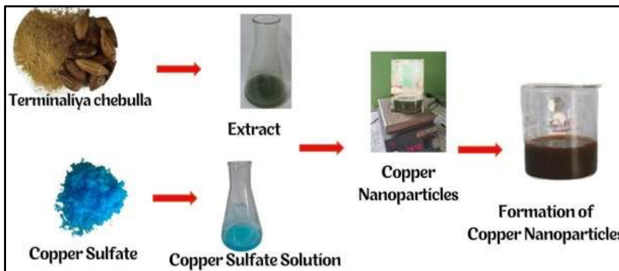
Figure 1. Schematic Diagram showing the synthesis of Coppersulfate Nanoparticles from Terminalia Chebula Linn Aqueous extract
