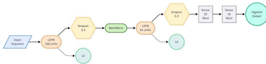
Figure 2. Regularized LSTM Architecture. Depicts dual stacked LSTM layers with dropout and batch normalization for temporal abstraction and generalization.
