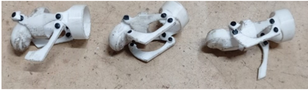
Figure 10: PLA Based Prosthetic with Broken Hinges caused due to Load Bearing Capacity Failure during Experimental Testing Trials
