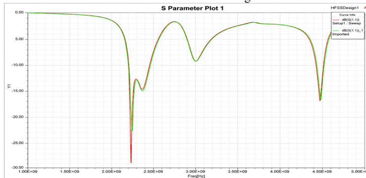
Fig 7. Comparison between Simulated and Measured Return loss S11 (dB) of antenna in free space
