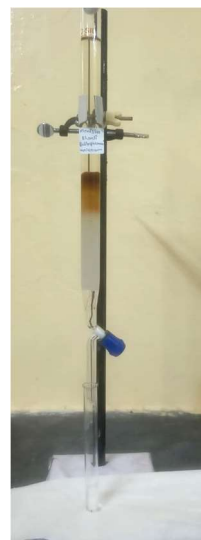
Figure 2: Isolation of active constituents by column chromatography
