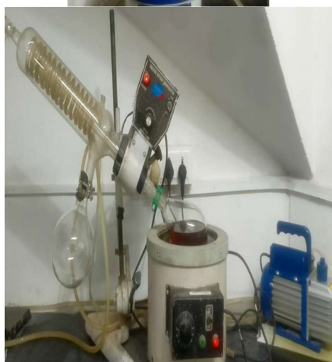
Figure 1: Soxhletation of Baliospermum montanum with Ethanolic Solvent
