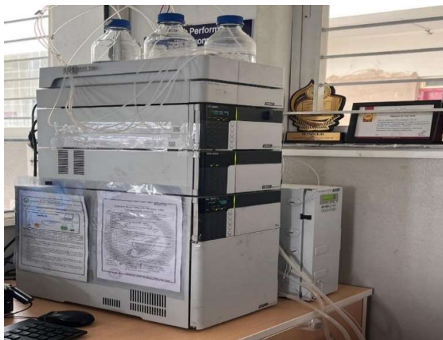
Figure No.3 Shimadzu HPLC system
