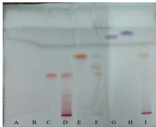
Fig. (2): Tracks A-Blank, B- Gallic acid, C and D- EGCG, E- Catechin, F-CS extract, G- Beta-sitosterol, H- Lupeol, I- BC extract at visible.
