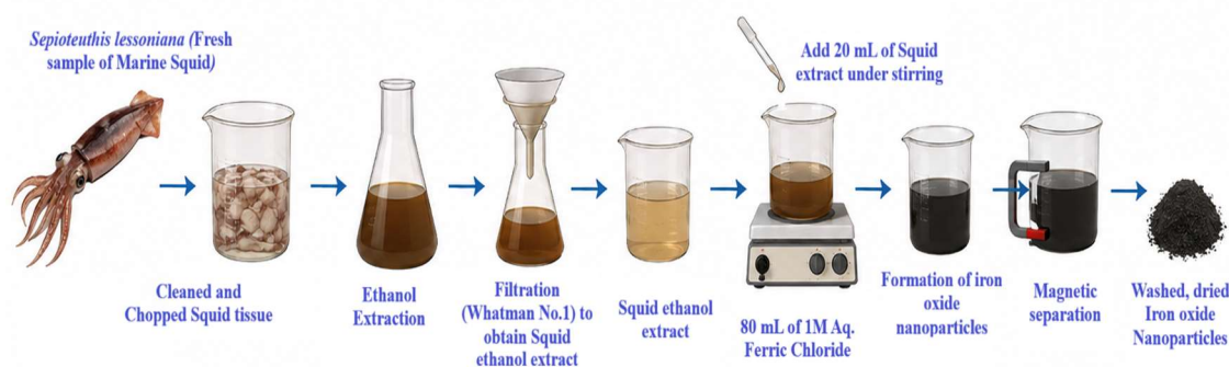
Fig. -2: Fabrication of Iron oxide NPs from Sepioteuthis lessoniana
