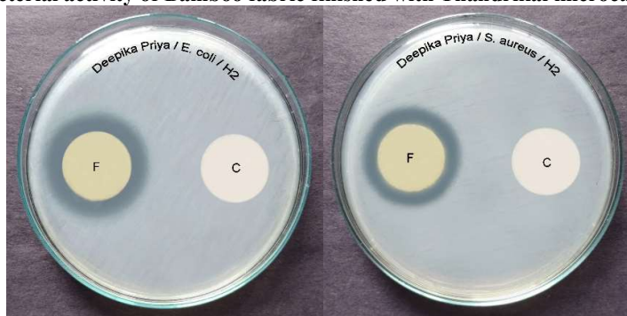
Fig. 3: Antibacterial activity of Bamboo fabric finished with Thandrikai microcapsules (BHM2)
