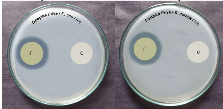
Fig. 2: Antibacterial activity of Bamboo fabric finished with Arasampattai microcapsules (BHM1)
