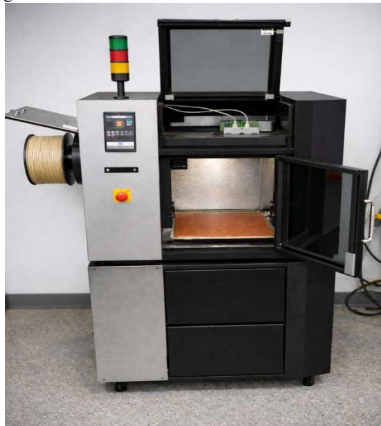
Fig. 2.4. High-temperature FDM 3D printer used for PEEK-based filament fabrication..
